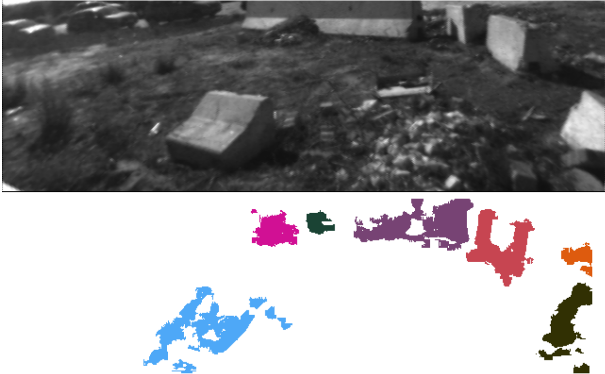
Fig. 3 – Stereo-based obstacle detection results. Each colour represents a different obstacle.
