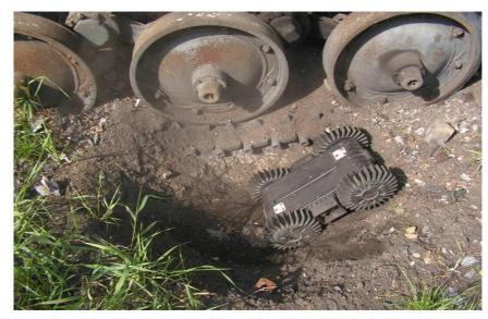
Superior terrain handling: thanks to the "Flapper Wheel" design (Pat. Pending) the unit is capable of handling extreme obstacles that can be impossible even for much bigger robots (the unit was tested in the EIRob Non-Urban scenario and managed to cross the "Potato Field" obstacle which proved fatal to several bigger competitors).
