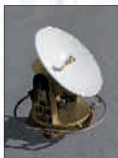
SatCom on the move terminal on top of the Gecko robot and the 90cm Satcom on the move terminal
