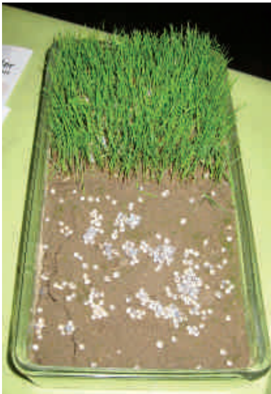
Mock up fluorescent biosensors used for detection in stationary display and possibly scenarios CRNE-Recon, consisting of Algin spheres of various diameters with fluorescent biosensor protein „tdTomato”
