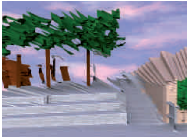
3D surface model from real LMS data, gathered in real-time with a low cost scanning system
