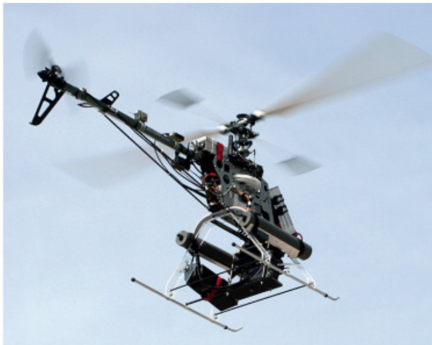
Autonomous Helicopter in flight with camera equipment underslung (Video in Youtube, look for „minihelicopter“ and „Offenburg“)
