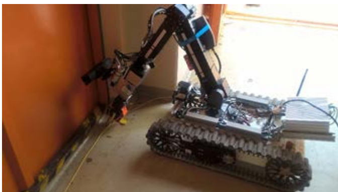
TAUROB Tracker in configuration “Reconnoitring of structures (3D mapping & find simulated radiation sources)”
